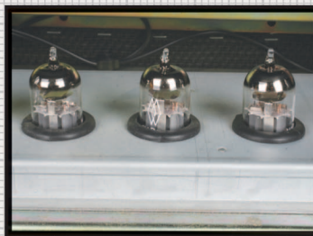
■ The front end of the Marshall with its new cryogenically-treated tubes
